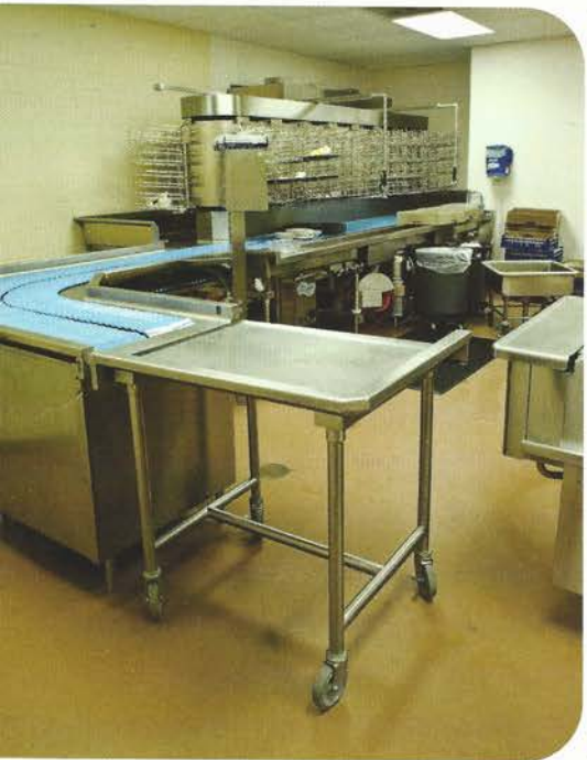
A multi-level tray accumulator (in background) ferries soiled dishes from Copper Grill directly into the dishroom.
